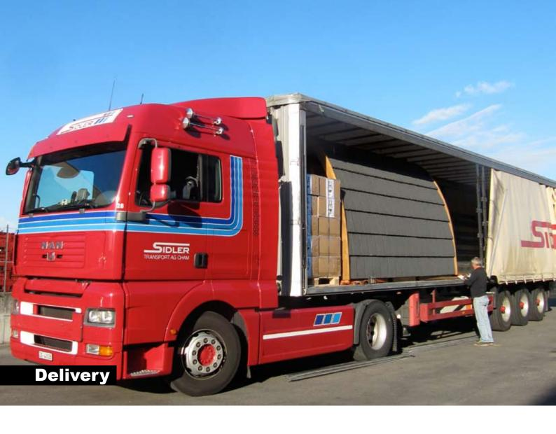
The PODhouses are delivered pre-assembled on a lorry. Thanks to the integrated steel rails, the PODhouses can be easily set down at the final site using a forklift with the necessary lifting load.
